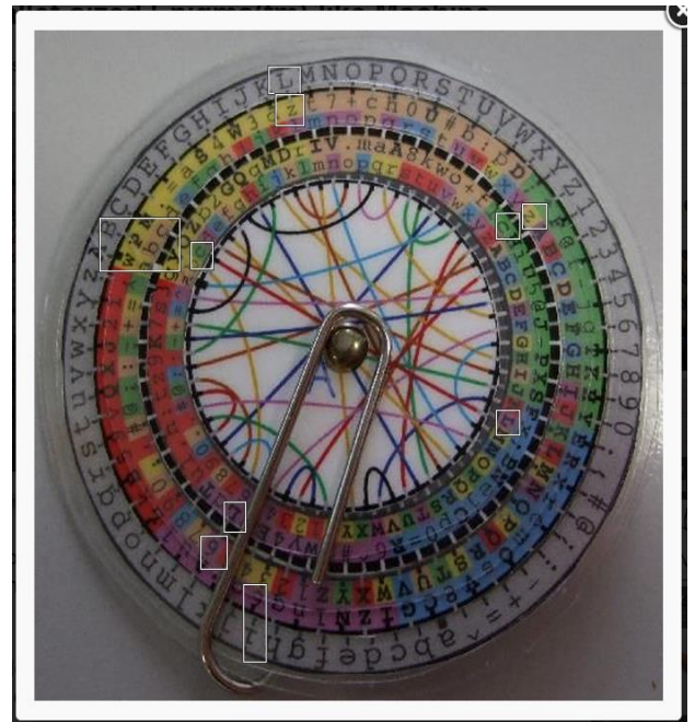
(A) Notice that with the rotors in the AAA position that the grey ticks of the two outer rings coincide? By noting this (or the opposite when it occurs), we are able to resolve ambiguous rotor transitions that can result due to off-centre rotors or general wear and tear. Refer to box (4) for a description of how this works.
